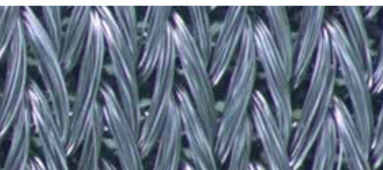
Each nylon strand is autocatalytically plated with 1 micron of 99.9% pure silver
